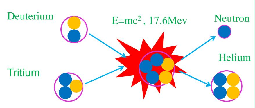
Out of 17.6Mev of energy, neutron takes 14.1Mev and 3.5Mev goes to α-particle
